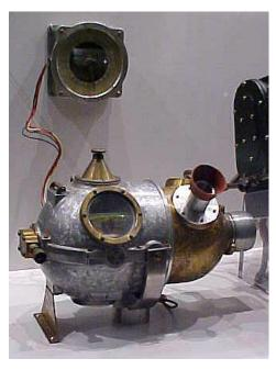
A new exhibit case, Military Avionics, is being installed in the north Aviation Hangar along the west wall (where experimental spacesuits were shown formerly). Radars, bombsights, and other exotic electronic devices are featured. One is the prototype Norden Mk XI bombsight from 1923 (photo, left), a device with a pleasing "steampunk" appearance. The installation will be substantially complete by the end of next week.
