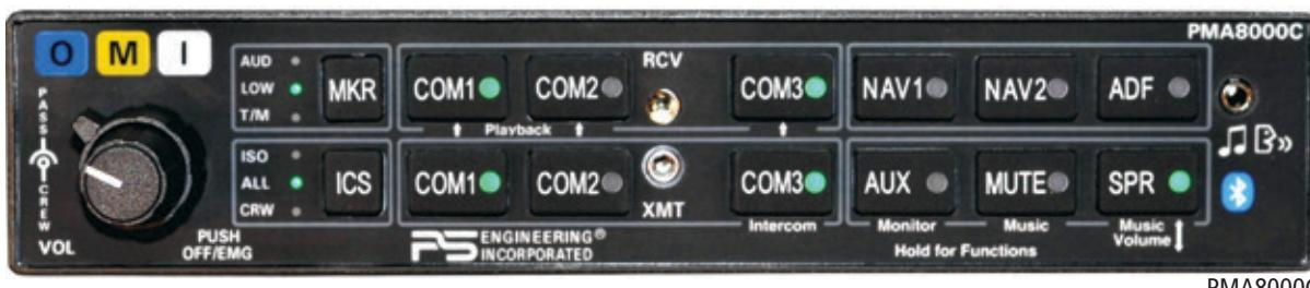
The PMA8000C provides for an additional communications transceiver. While most aircraft have two Com radios, there are cases where a third transceiver is required. The PMA8000C not only allows the connection of three radios, it also provides 3 unique split transmit modes.
