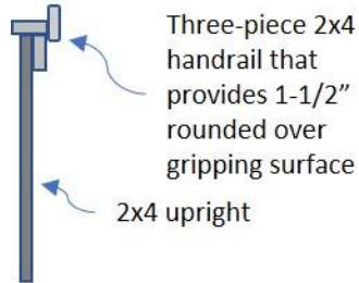
Pros: Provides a near continuous 1-1/2" wide rounded edge gripping surface with most of the end grain protected from weather.
