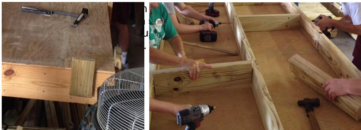
The interior area of this jig is left completely open which allows for custom module lengths and easy changes to the module structure as new approaches are identified or custom needs arise. Standard locations for the interior boards can be marked directly on the plywood to speed assembly. Note that this design even allows for building modules with the lumber "flat" to create a 1 1/2" thick module as opposed to "on edge" for a
