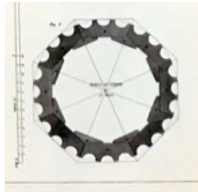
Half of Plate XXIV, titled "Glueing up of Columns" in The Architect, or Practical House Carpenter , by Asher Benjamin, 1830.
