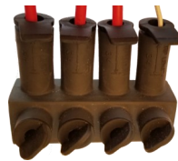
270RC4 Re-enterable Connector waterproof wire sleeves, 4 connection lugs, 2/0 to 14 AWG copper or aluminum wire (2, 3, 6 connector versions available)
