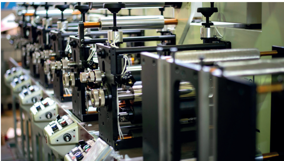
The Brazilian-built six-colour Etirama Superprint UV and hot air press.
