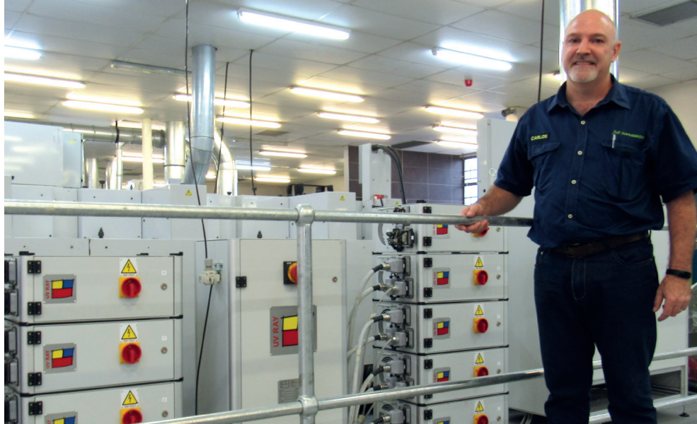
FIL's production manager, Carlos Mangos, in front of the Atom UV ink curing system from Italy's UV Ray, which has been retrofitted on a 10-year-old Mark Andy 22000 H series press.
