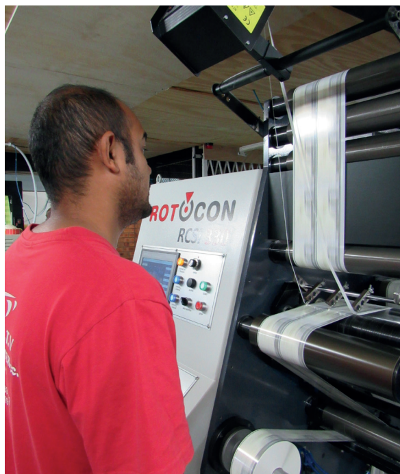
The LED strobe light in the vertical inspection zone, automated tension control and self-explanatory icons on the moveable operator console, make the Rotocon Ecoline RCSI 330 finishing machine simple to operate.
