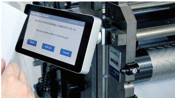
Wink's SmartGap AutoControl feature continuously monitors the die-cutting result and automatically adjusts the cutting depth
