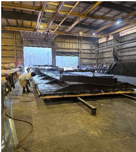
The chassis and floor system are shown early in production. Attendees observed the floor assembly inverted while the bottom subfloor, ductwork, plumbing and other concealed components were installed before the assembly was turned upright and construction continued.
