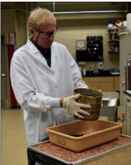
Bahr is analyzing a sample of gravel and reclaimed asphalt from a road in Cass County.
