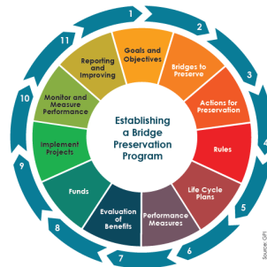
Figure 15. Steps for establishing a bridge preservation program.
