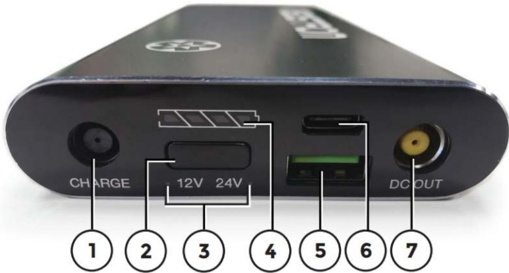
1. **Charge Port:** Plug the compatible AC adapter into this port (use the short charging adapter cable if required). Ensure that the AC adapter is plugged into the main power outlet. Once the battery is charging the 4 green Charge Level Indicator Lights will turn on.
