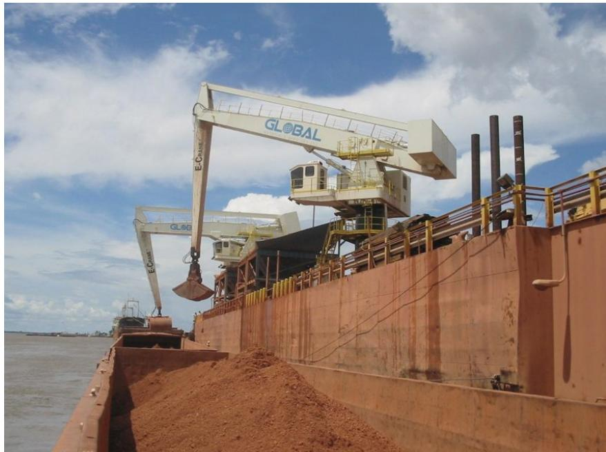
In 2002 and 2003, two E-Cranes were installed at Global Materials Services in Venezuela. Both material handling E-Cranes are installed on a floating platform on mile 182 of the Orinoco River in Puerto Ordaz. The E-Cranes unload barges of bauxite into two hoppers also mounted on the floating platform.
