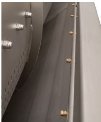
Washing ramp for pierced tank SPO open-cage presses
