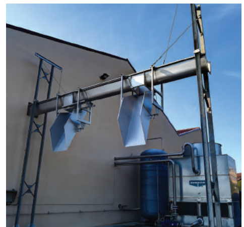
Pomace removed by conveying screw with carrier and duct system for filling poly-bins - pneumatic control of ducts and hatches
