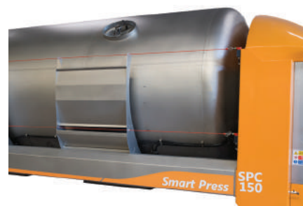
Technical access hatch to tank on air side
