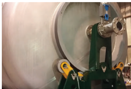
Hardy design: Smart Press 480 – 600: the press cage is set on two bogies
