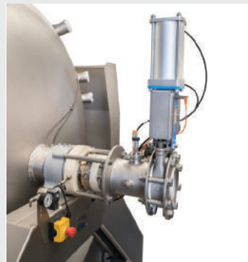
Axial feeding with pneumatic valve
