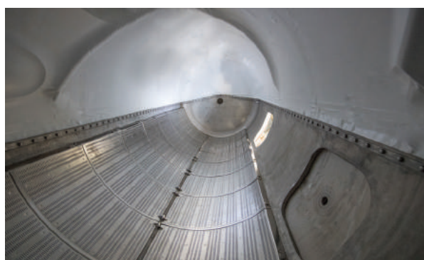
Closed cage from 20 to 600 hl Fast Press grids = better drainage and easier washing
