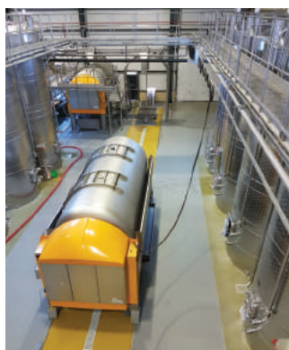
Motorised press travels on rails
