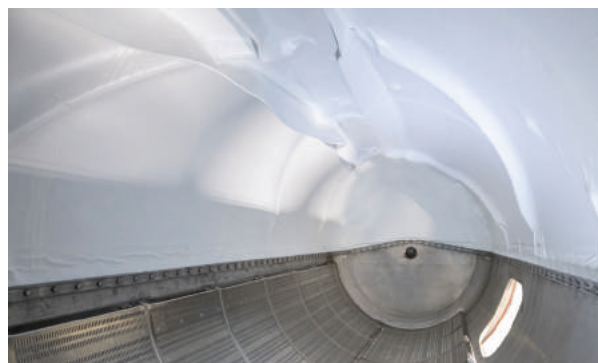
SPC - Pomace drainage coils
