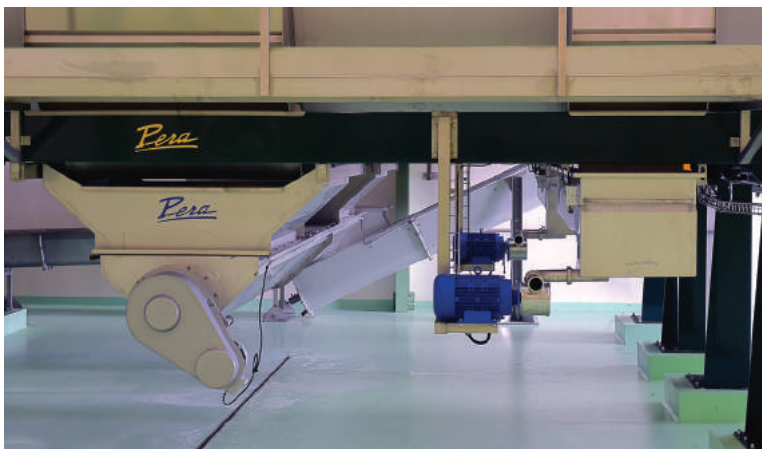
Pomace removed by conveying screw with carrier and duct system for filling poly-bins - pneumatic control of ducts and hatches
