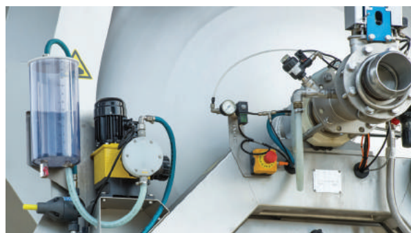
ENOXY + system (Vat and dosing pump for the antioxidant solution)
