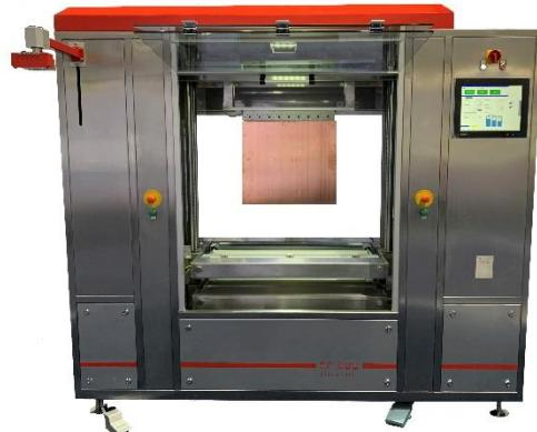
One of the most important and most frequently expressed wishes is to significantly minimize the contamination of operating personnel with the filling paste. This means that the handling step of manually moving the freshly filled panel into the cleaning chamber must be avoided. As a result, we now have a combined filling and cleaning chamber in this new system. The cleaning takes place automatically - immediately after the filling process.
