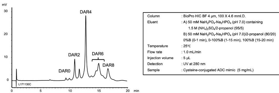
The BioPro HIC BF column shows superior resolution compared to competitors' columns and is highly effective for determining drug-to-antibody ratios of Antibody Drug Conjugates.
