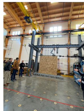
From the archives, the SEAW SW Chapter toured the APA testing facility in April 2023, where they saw a full-scale shear wall test in progress. Photo by Jacob Baker.
