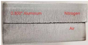
Use of high or low pressure dry air can greatly improve edge quality when laser cutting aluminum.
