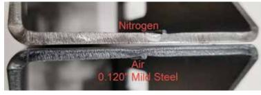
In laser cutting of mild steel, the choice of air or nitrogen depends upon material thickness, cost considerations and finishing.
