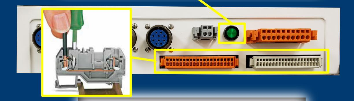
Positive latching Wago Cage Clamp® Connectors help prevent wire release due to vibration.
