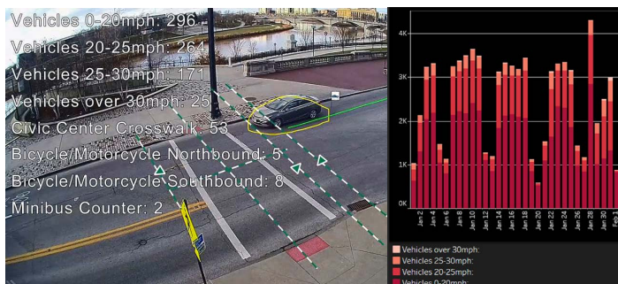
Programming cameras to track vehicle counts and speeds can provide meaningful data.
