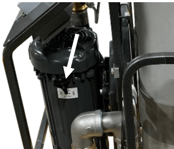
On/Off Switch located directly on the motor
