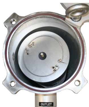
Cartridge Housing with Coalescer Cartridge and Water Separator Filter in place with Retaining Washer
