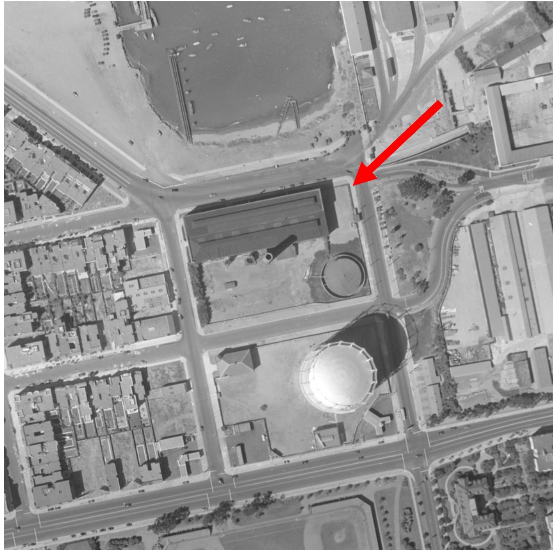
Figure 12: 1938 Aerial Photograph Harrison Ryker, Continues to show multiple oil tanks on the site. Source: David Rumsey Maps.
