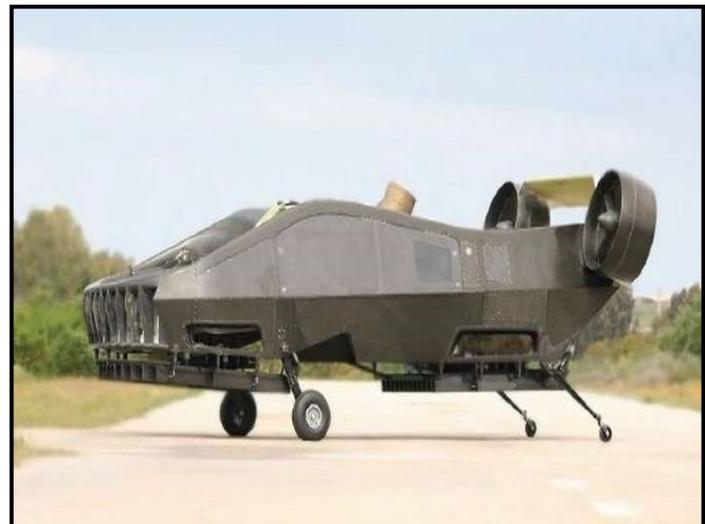
The robotic flyer pilots itself entirely through laser altimeters, radar and sensors. The system is "smart" enough to self-correct when it makes mistakes, company officials said. In a video released by Urban Aeronautics, the Cormorant tries to land, stops itself and then corrects its landing position.
