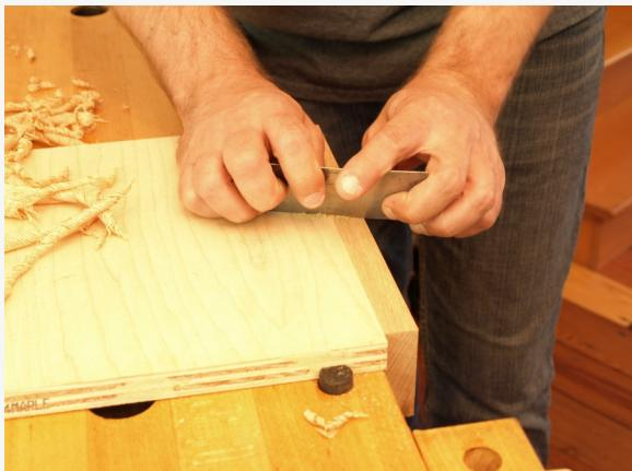
*If I keep my weight on the rear of the plane during the cut, it will keep taking shavings off the edge band until it is flush with the plywood, and then be unable to cut any deeper. I can usually clean up about 90 percent of the edge band this way. But If the plywood isn't totally flat, there may be a few spots to touch up with a card scraper before sanding.*
