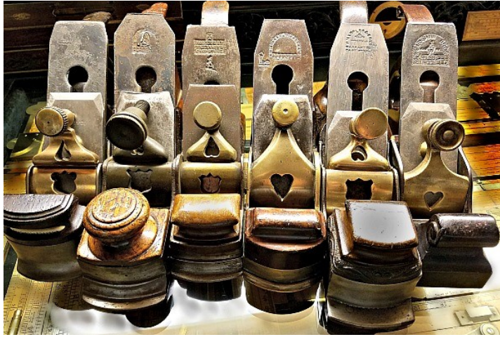
Above: 6 different 19th Century Scottish handplanes with pierced lever caps, illustrating Scottish style piercing discussed here by bill. Thank you to collector George Anderson. You can reach George at sgando99 on Instagram.
