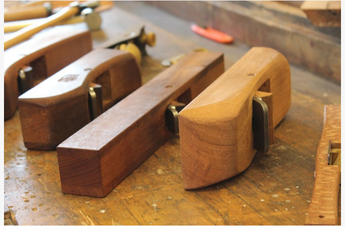
Student made wooden handplanes at Etz Ladaat . Different shapes and sizes to fit each hand and working style.
