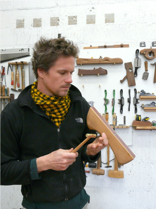
Nathan Van't Hof instructs students on adjusting the blade in their Krenov styled wooden handplane at Etz Ladaat School of Fine Woodworking .
