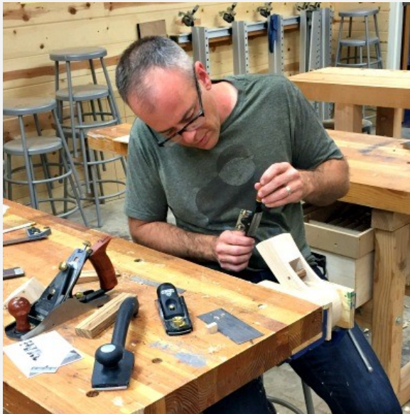
Using a metal plane to get the wooden hand plane's shape just right at Southwest School of Woodworking .
