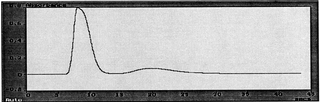
The two individual peaks correspond to the two absorbance cells of different sensitivities. The maximum intensity of the long pathlength cuvette (low range cell) occurs at ~8 sec and the maximum intensity of the short pathlength cuvette (high range cell) occurs at ~20 sec.
