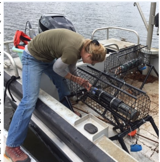
Pictured above: Natural Resource Biologist prepares an automated water quality meter for deployment into Deep Creek Lake
