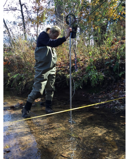
Above: Natural Resource Biologist measuring water velocity and depth along a cross-section of a lake tributary as part of the tributary monitoring effort
