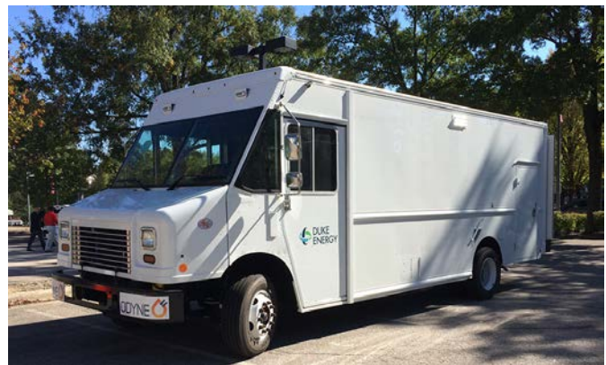
Duke Energy work truck equipped with the Odyne plug-in hybrid system
