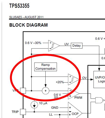
DCAP2/3 conditions the FB signal introducing delays
