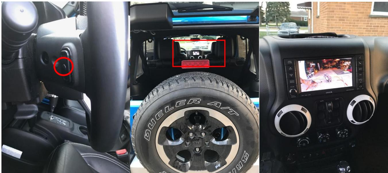
18. To activate the Navigation Unlock, Hold the Source button (behind the right side of the steering wheel). Your LED will begin to blink. Press it one more time to confirm "passenger presence" – LED will go solid and Nav will
