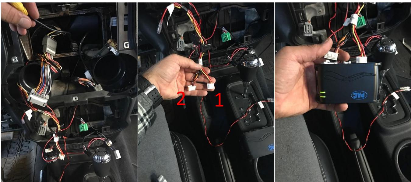
16. With everything working, tuck the BCI interface module into the open space next to the driver side vent (Blue circle) Then connect the black and red wires to the LED (they are clearly labeled. I taped them as well. I did not use the small red wire labeled "Camera power output". Then carefully tuck the camera power wires and LED wires down and out of the way then replace the HVAC panel. Be sure to reconnect all of the plugs!
