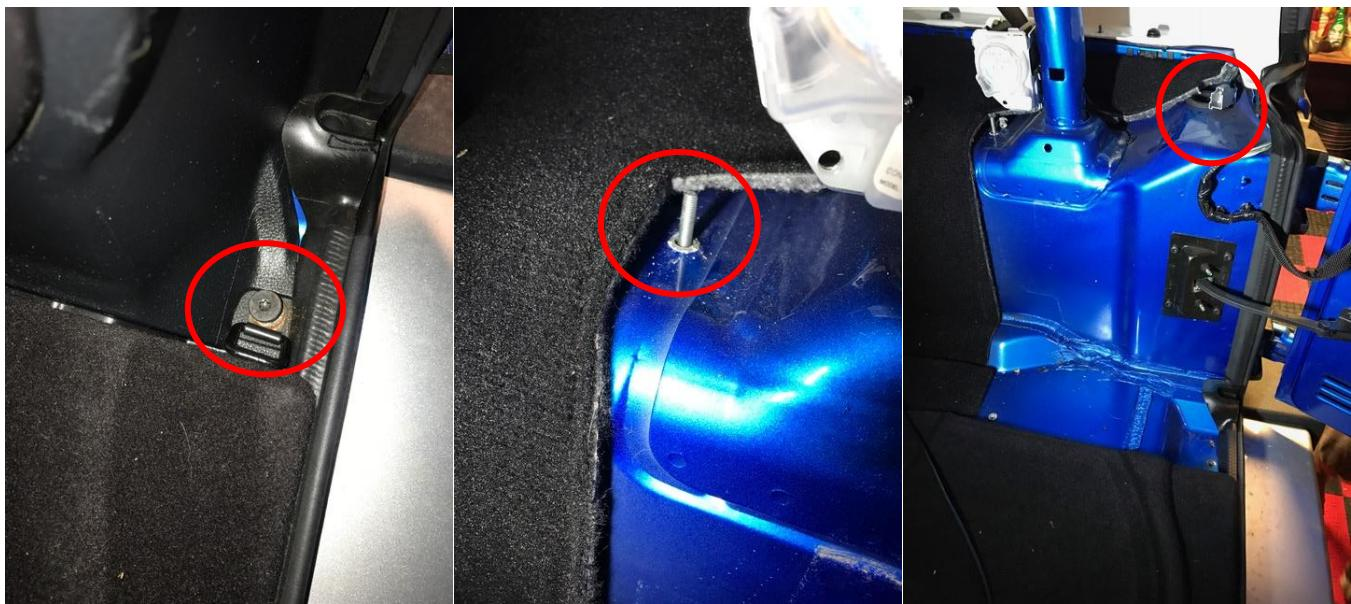
6. I chose to remove some of the zip tie/ Christmas tree fasteners that are used to keep the wires in place. If you cut them off and remove the loose piece and extra tab, you can feed your own ziptie through it and reinsert the Christmas tree fastener into the hole!
