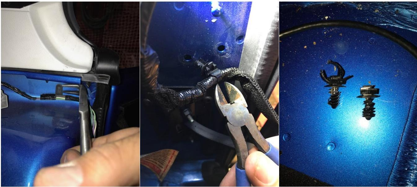
7. Pull back the carpet from the rear corner of your passenger side and then work forward removing the B pillar plastic clips (4). My angled needle nose worked best for these. You don't have to remove the bottom of the B pillar, there is enough room to safely run the cable and sneak the passenger floor panel out from underneath it.
