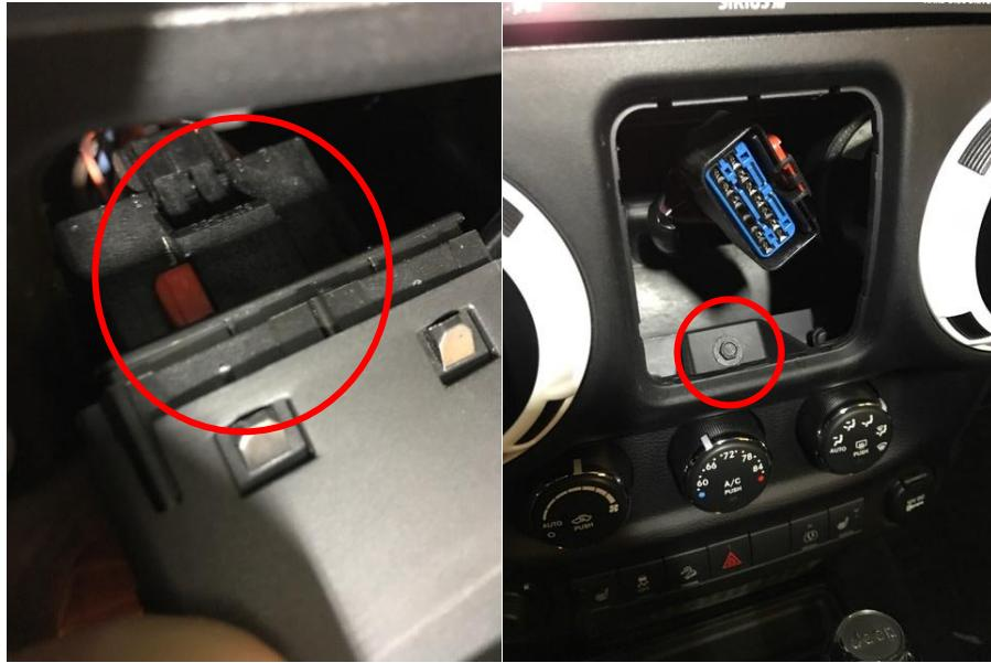
3. With the dash removed, Remove your stock radio by removing the 4 – 7mm screws at the four corners and pull the radio toward you. You will need to remove the plugs from the back. Then carefully pry the HVAC panel toward the center of the vehicle to pop it out. Once free you will need to reach in and remove all of the harnesses attached.
