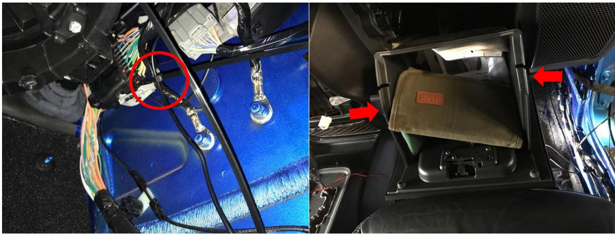
11. Bring the cable through the glove box toward the center counsel. There is a small passage you will be able to feed the yellow RCA & small black and red wires through. Route the Yellow RCA wire behind the plastic panels up to where the window switches are (3<sup>rd</sup> pic).
