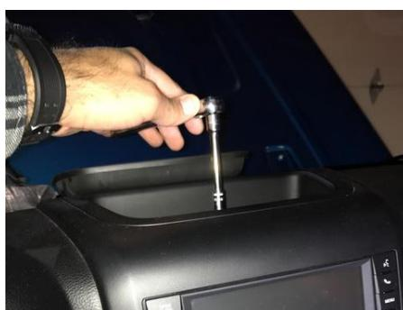
b. Remove the plastic kick panel below the steering wheel by pulling toward the driver seat and down from under the steering column. There are 4 tabs in the 4 corners & hinges at the bottom holding it on. Then Remove the two 7mm bolts located at the top on both sides of the steering wheel (circled)
