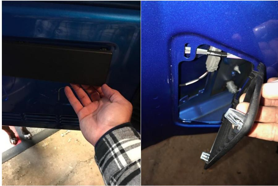
5. My vehicle is equipped with the factory subwoofer so that panel needed to be removed. Two T-30 Torx bolts & and 10mm bolt near the seat belt/ roll cage to tub on top. Once free remove the plug.
