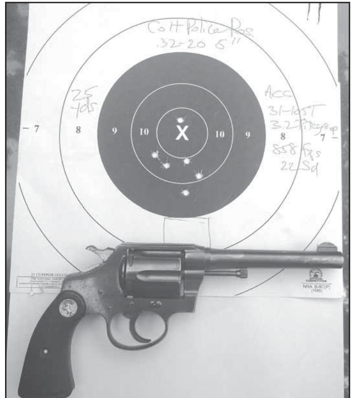
A good load for the Colt Police Positive with the Accuracy 31-105T was 3.2 grs. of TiteGroup
