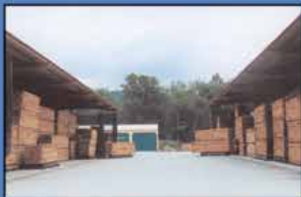
Lumber stored under T-sheds.
