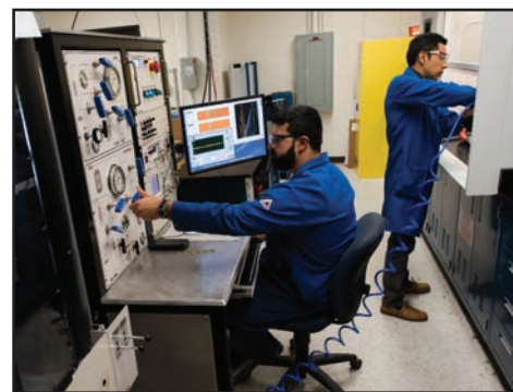
Principle Investigator for the Energy Applied Geomechanics Laboratory, Dr. Nicolas Espinoza (right), and Ph.D. student, Matthew Ramos (left), acquiring real-time ultrasonic measurements at reservoir conditions using the group's state-of-the-art triaxial load frame (Photo courtesy of the Department of Petroleum and Geosystems Engineering at The University of Texas at Austin).
