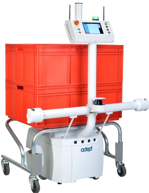
The Adept Lynx® Cart Transporter is an Autonomous Intelligent Vehicle (AIV) designed to attach to moveable carts and transport them from a pickup location to a drop off location. Applications include line-side inventory replenishment, moving flow racks, transporting Work in Progress between process steps, and moving finished goods to the warehouse.
