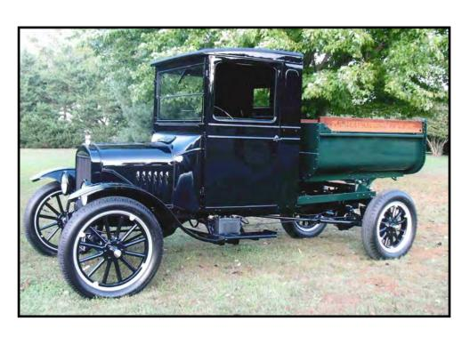
The second "T" in the Model TT truck indicates that it is the one-ton version of the Model T truck which was built from 1917 to 1927. The truck had a longer wheelbase (125") than the Model T car (100") and was fitted with a sturdy worm-gear rear axle.
