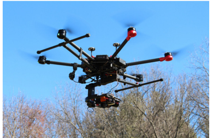
The DJI Matrice 600 Pro is a professional-grade VTOL platform for hyperspectral remote sensing missions
