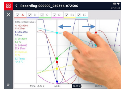
Figure: Using the magnifying gesture with two fingers, the operation is carried out – zooming in this case
