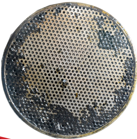
Dirty Pump Screen - Conventional CJ-4
