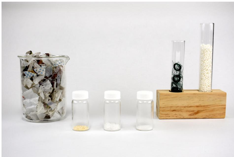
Hard-to-recycle plastics (left) are used to create chemical compounds (center) suitable for making automotive parts, apparel, electronics, paints and coatings, solvents and even fragrances (right).
