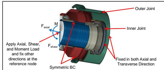
b) Boundary conditions applied on Engine Line Flex Joint 3-D FE model for combined load condition.
