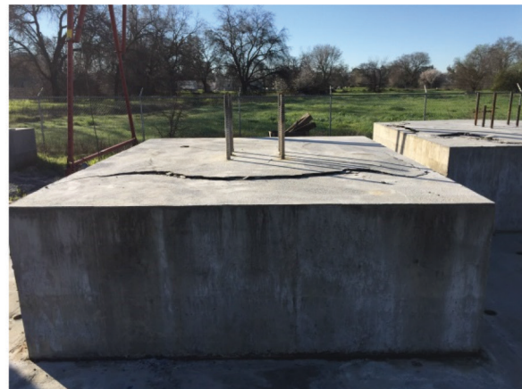
Fig. 6. Profile view of breakout surface: (a) 12-in. embedment; (b) 18-in. embedment.
