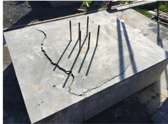
Fig. 5. Overhead view of breakout surface: (a) 12-in. embedment; (b) 18-in. embedment.
