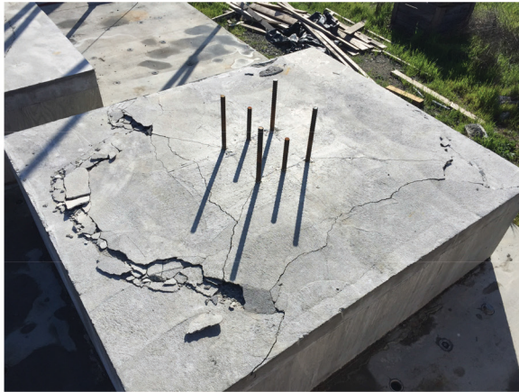
Fig. 5. Overhead view of breakout surface: (a) 12-in. embedment; (b) 18-in. embedment.
