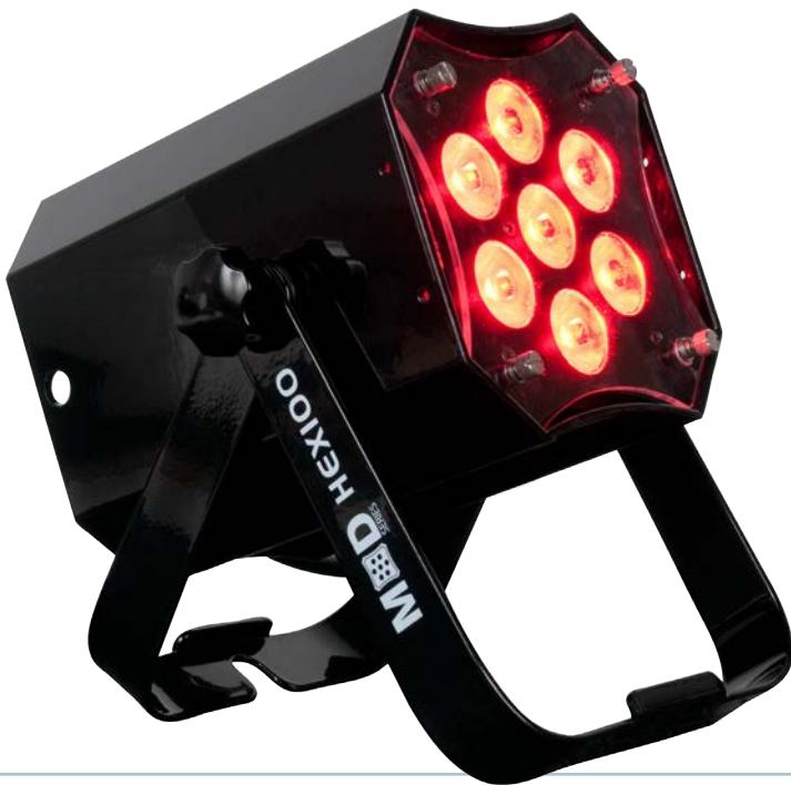
The MOD HEX100 comes equipped with seven 15-Watt RGBWA+UV (6-IN-1) LED diodes (for a total output of 105W), a scissor yoke and three interchangeable frost filters that are easily replaceable by thumb screws. The 17-degree standard beam may be changed on the fly to 20, 40 or 60-degrees.
