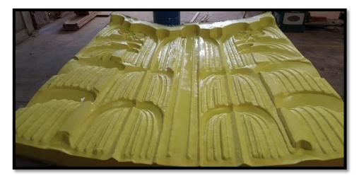
From these refurbished pieces, our team was able to create a rubber mold, with a fiberglass mother mold, to ensure that everything held its true shape. We were then able to cast new panels.
