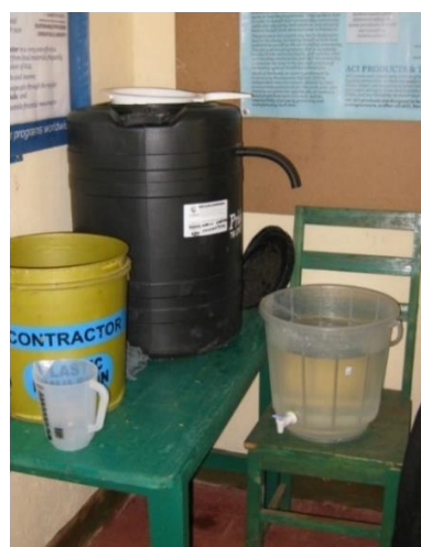
ACK demonstration plastic biosand filter (2011)
