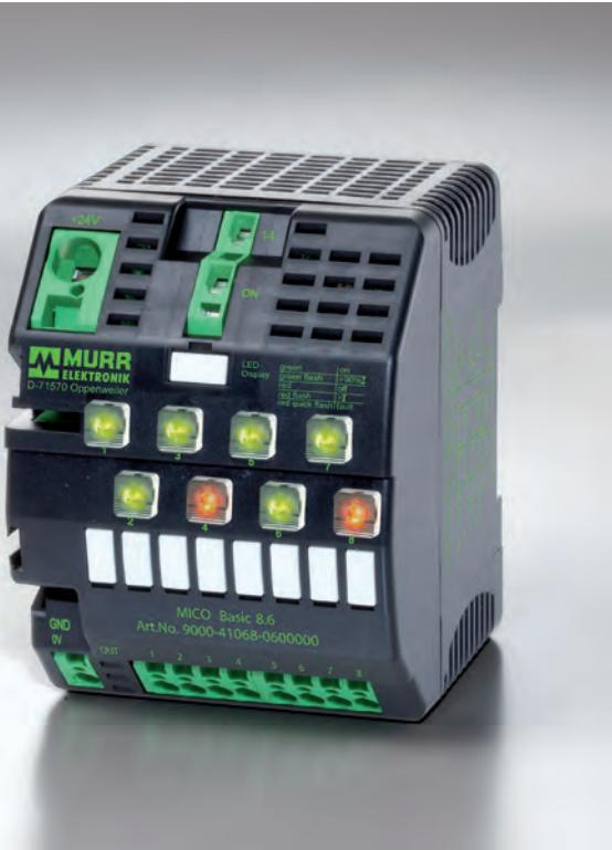
MICO eliminates start-up peaks with a time-delayed (cascading) start of individual current paths. Advantage: Now you can use power supplies with lower output current.
