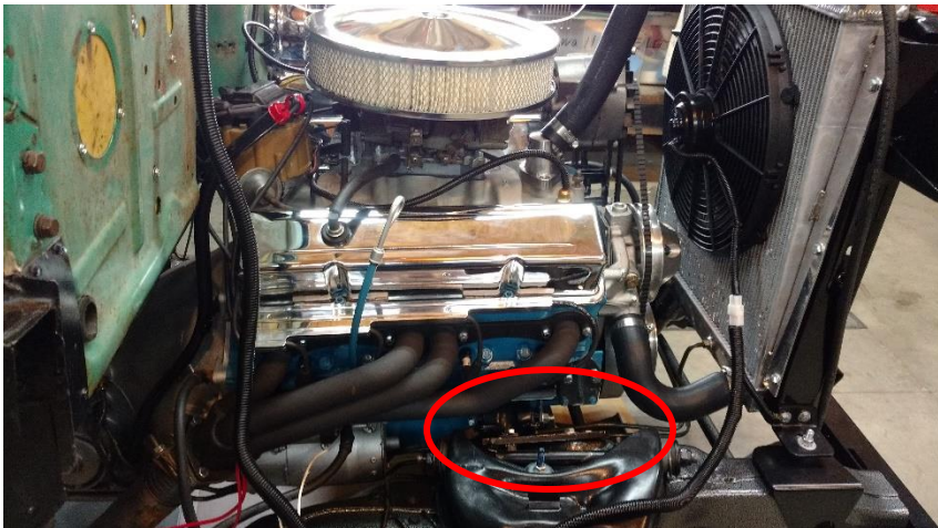
Passenger side of engine, moved back towards the firewall using the set back plates in the Grand Slam engine mounts. (circled in red)
