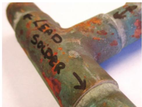
Lead leaching into the drinking water is not limited to lead pipes. Lead contributors, such as leaded solder in copper piping systems used until 1986 as well as brass valves and fixtures, can leach lead at levels that exceed the EPA's cut off levels. Even with an awareness of the health dangers of lead, the term Lead Free, until 2014, included plumbing fixtures that contained as much as 8 percent lead.
